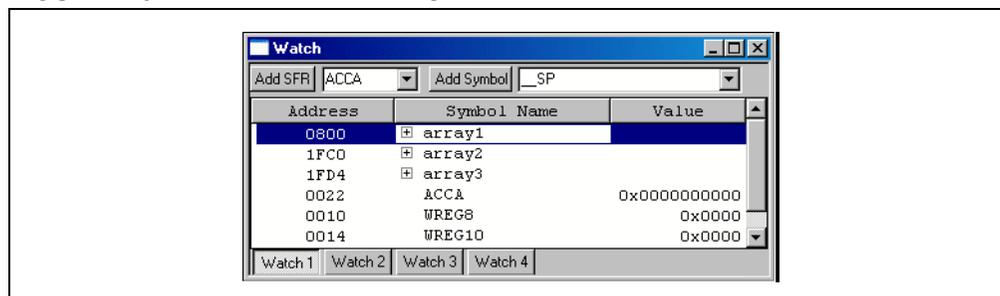
Click on the plus symbol to the left of the symbol name to expand the arrays. At this point in the program, both `array1` and `array2` should have been set up with initial values, but `array3` should be all zeros, since the `modulo()` routine has not yet been called.
