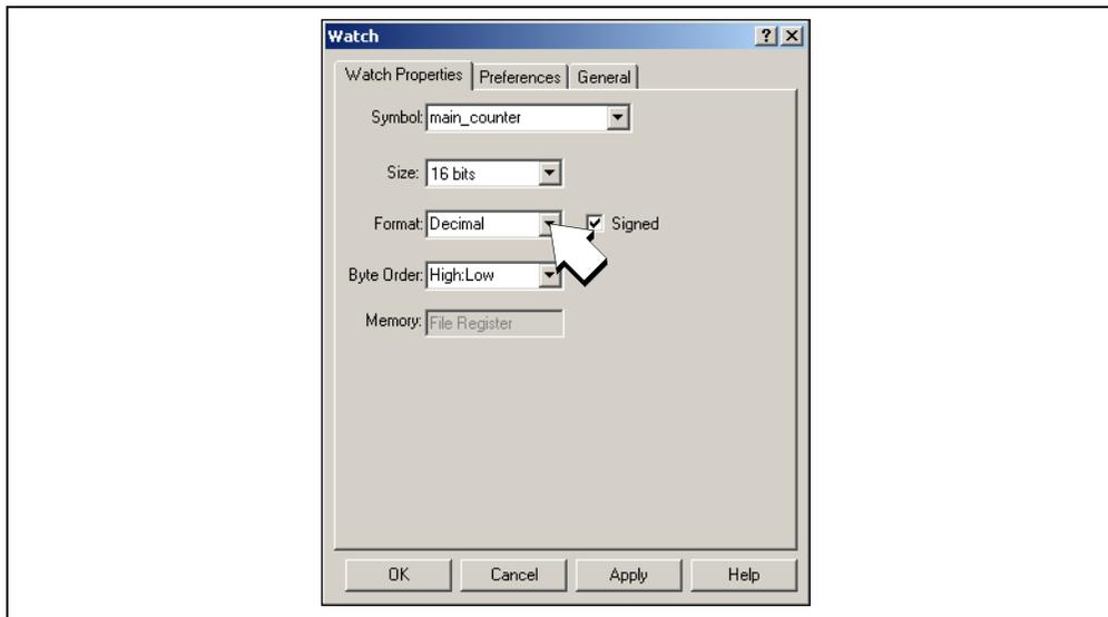
The `main_counter` value should now show 1000. Press the Step Into icon a few more times to see the changing variables, especially `sticks` and `irq_counter`, which are incrementing each time the interrupt happens.
