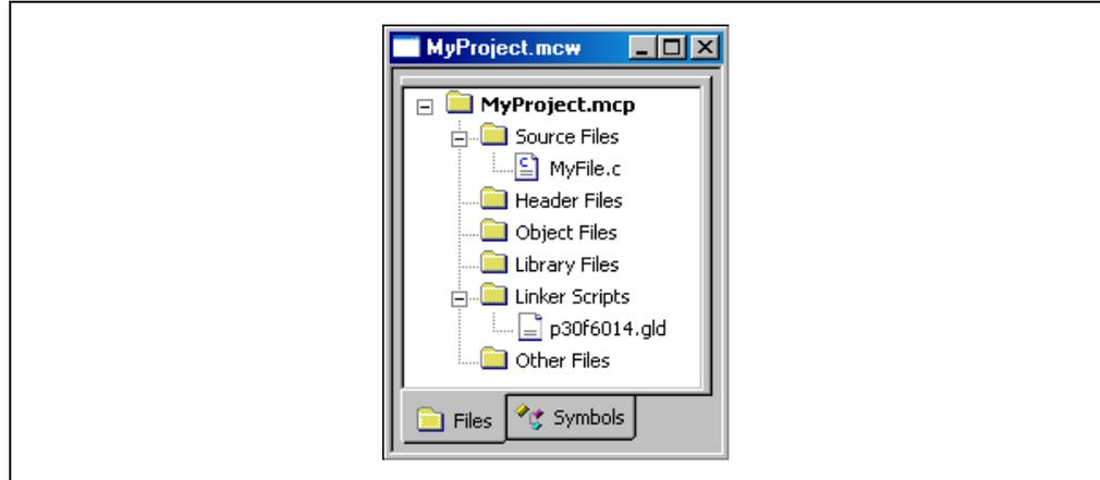
**Note:** If an error was made, highlight a file name and press the Delete key or use the right mouse menu to delete a file. Place the cursor over “Source Files” or “Linker Scripts” and use the right mouse menu to add the proper files to the project.
