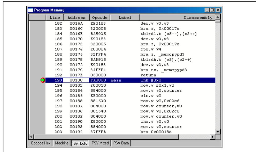
5. Go back and look at the source file window (*File>Open*) and the Disassembly window (*View>Disassembly Listing*). The breakpoint should be seen in all three windows. The step function can now be used in any window to single step through C source lines or to single step through the machine code.
