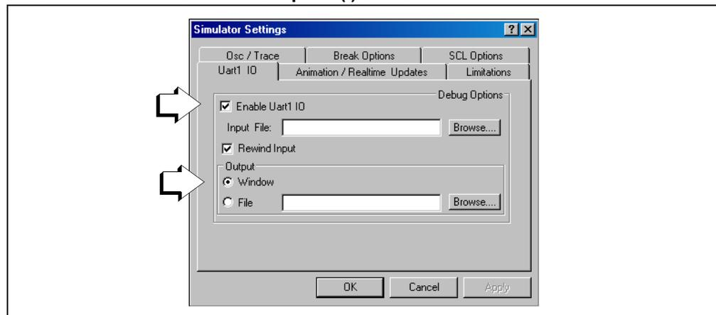
Now recompile your project (*Project>Build All*). Press Run, let it run for a few seconds, then press Halt. If the output window is not present, enable it on *View>Output*. Click the **SIM UART1** tab. A log of the contents of `array3` should have been generated in the output window.
