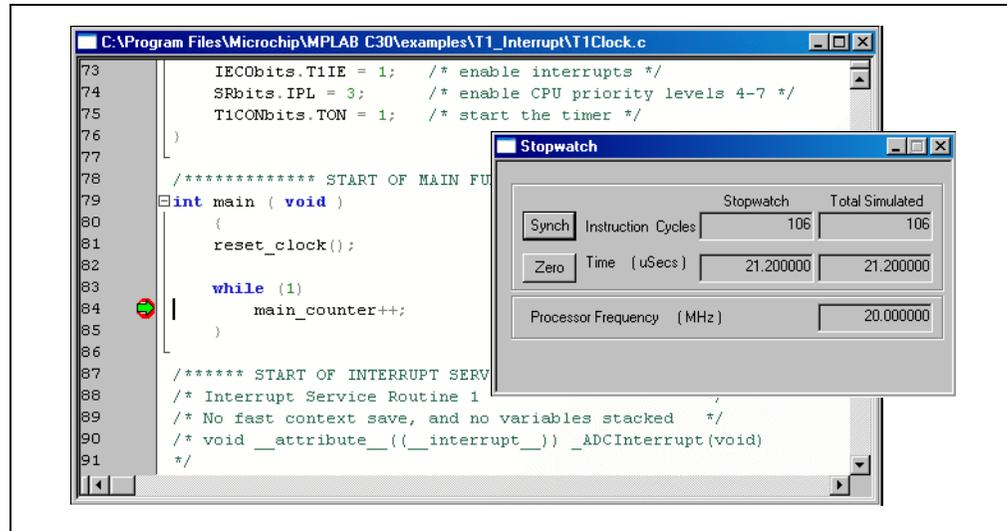
If the run was successful, then a Watch window can be set to inspect the program’s variables. Select *View>Watch* to bring up a Watch window. Add the variable `RTclock` (from the drop-down box next to **Add Symbol**.)
