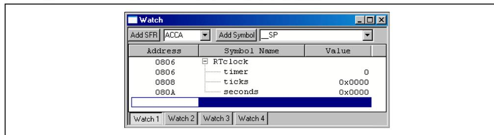
In addition to `RTclock`, add the variables `sticks`, `irq_counter`, and `main_counter` to the Watch window.
