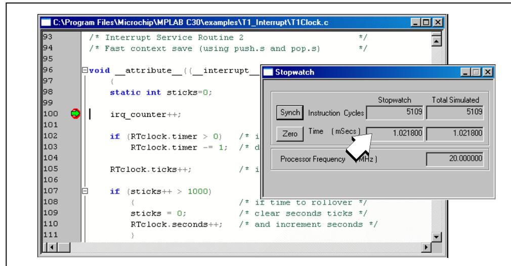
The value shown in the Time window is 1.0218 ms. This is about what was expected, since the interrupt should happen every millisecond. There was some time since Reset that was counted by the Stopwatch, including the C start-up code and the Timer 1 initialization.
