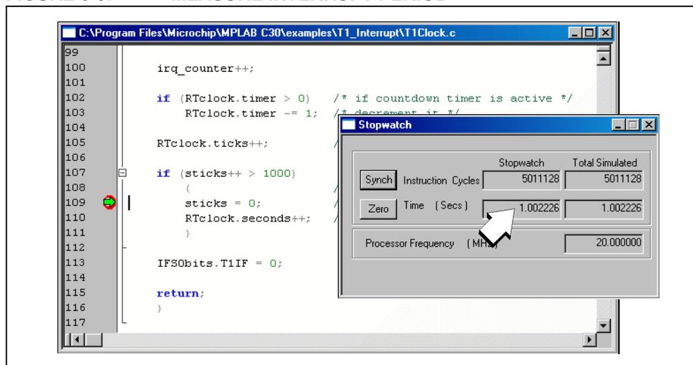
The Stopwatch Time window shows 1.002226 seconds, which is close to a one second interrupt. A good time measurement would be to measure the time to the next interrupt. That value could then be subtracted from the current time. Or, since it doesn't matter how much time it took to get here – the main interest is the time between interrupts – press Zero on the Stopwatch and then press Run.
