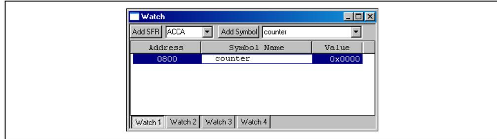
**Note:** There are three ways to enter Watch variables: (1) in the method described above, a variable can be picked from a list, (2) the symbol's name can be typed directly in the Symbol Name column in the Watch window or (3) the variable's name can be highlighted in the source text and dragged to the Watch window.
