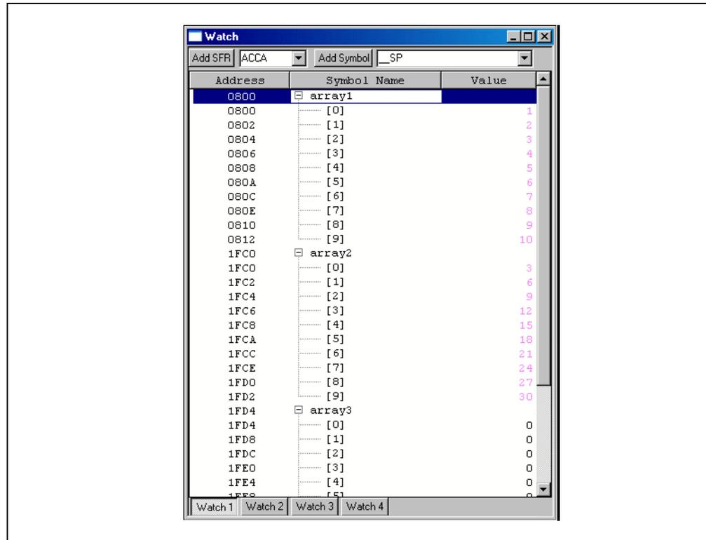
Set a breakpoint in the `modulo.s` file at the start of the `DO` loop. Run to the breakpoint and scroll the watch window to look at `array3`. It should still be all zeroes.
