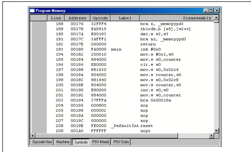
By selecting the various tabs at the bottom of the Program Memory window, the code can be viewed with or without symbolic labels, as a raw hex dump, as mixed PSV code and data, or just as PSV data.
