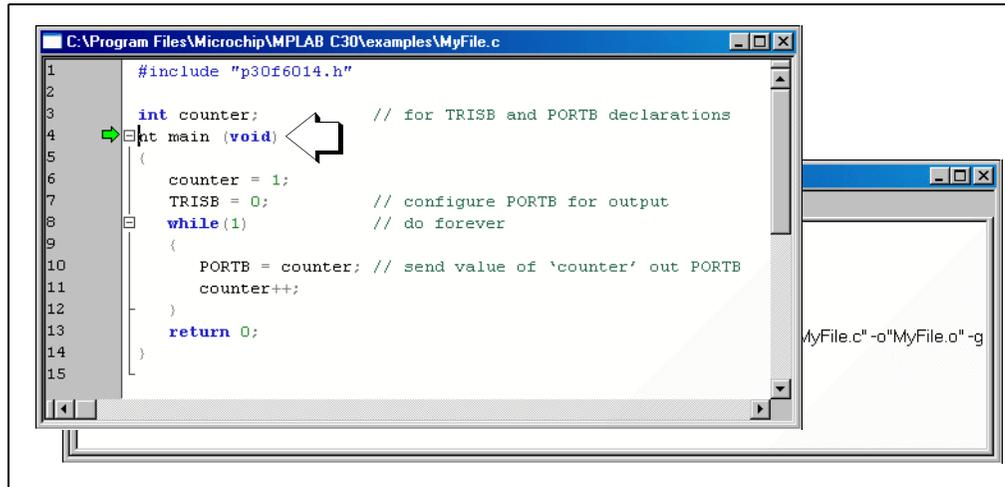
The offending typo “nt” is in black text rather than blue – a good indication that something is wrong, since key words are shown in blue color fonts. Typing an “i” to make the “nt” the proper key word “int,” results in the text turning blue. Selecting *Project>Project Build All* again produces a successful build.
